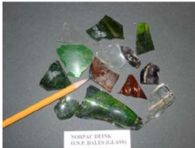
Figure 24: Glass collected in commingled recycling programs can end up at paper mills and seriously damage paper-making equipment. This 2009 photo shows glass that was in a paper bale and rejected in the pulping process at NORPAC.
